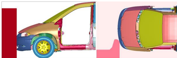
Fig. 17 The SOFI full vehicle model pre-crash
